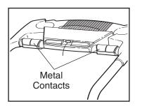
To measure your heart rate, **stand on the foot rails** and hold the metal contacts on the pulse handgrips—**avoid moving your hands.** When your pulse is detected, the heart symbol in the Pulse zone of the display will begin to flash each time your heart beats, one or two dashes will appear, and then your heart rate will be shown. For the most accurate heart rate reading, continue to hold the contacts for about 15 seconds.
